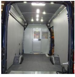
DuraTherm consists of dual polypropylene outer skins, vacuum heat sealed to a central honeycomb plastic core, resulting in a 5/16" thick panel. A foam/foil insulation is then added to the back of the panels to get the perfect interior liner product. All pre-cut, pre-drilled sections are extremely lightweight.
