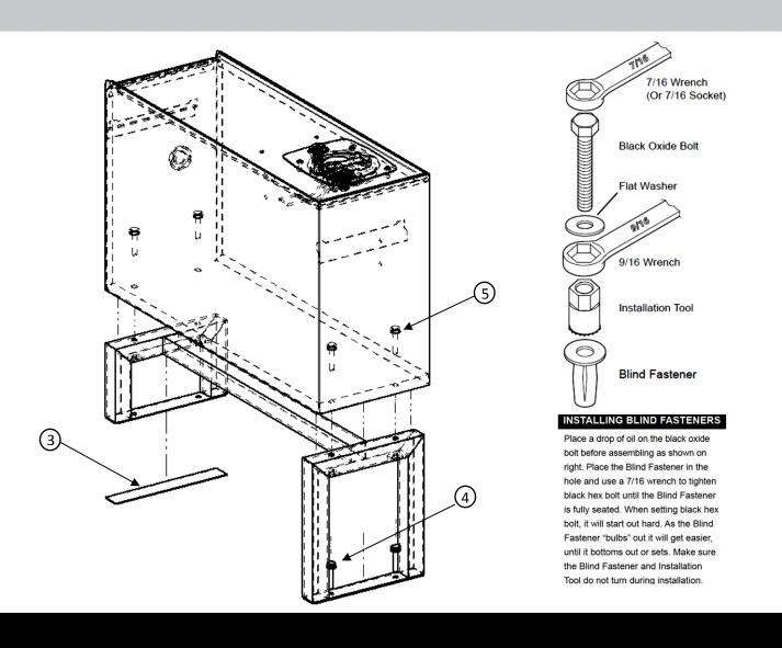
**STEP 1.** Position mounting base in cab between seats being careful not to place over grounding wire and and mark the location for the mounting bolts in the rear mounting foot.
