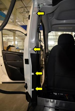
2.10. Bring partition into the vehicle. (It can be half-assembled if installed by only 1 person)
