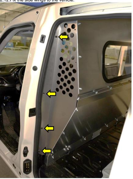
2.13.Install the missing bolts and tighten every fastener.
