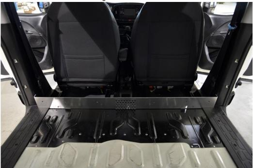
2.5. Install two fasteners in the middle of the bracket. Do not tighten yet.
