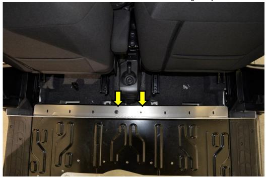
2.6. Assemble the side wings with the lower panel as per drawing.
